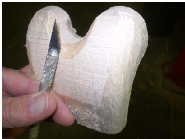
Round the edges with an X-Acto knife and sanding tube per the full-size photo.
