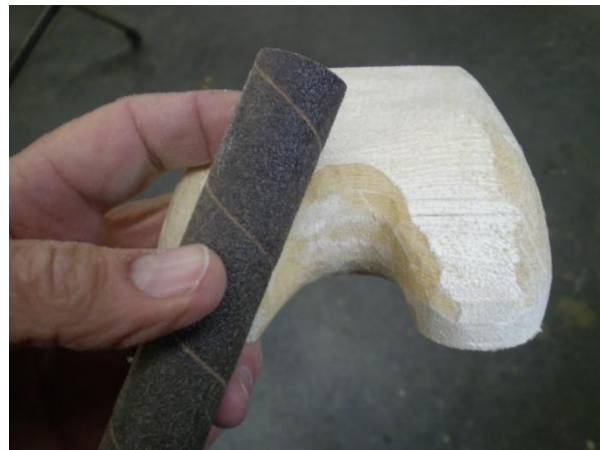
Round the edges with an X-Acto knife and sanding tube per the full-size photo.
